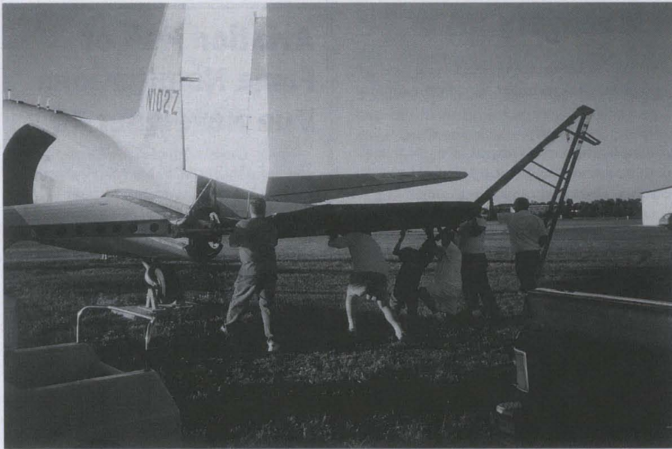
DTAM volunteers recently got together to help remount the Museum's Douglas C-47's control surfaces. The surfaces had been re-covered and were placed back on "the old-fashioned way."
