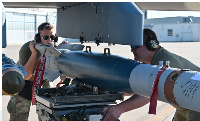
119th Wing weapons load a GBU 12 missile on an MQ-9 Reaper prior to a mission in support of Exercise Hawkeye Fury at the Iowa National Guard base, Des Moines, Iowa, Sept. 19, 2022.
