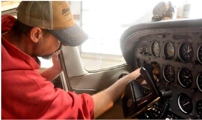
Lancaster Avionics technician Scott Kuhns installs a FreeFlight Systems UAT control head in a Cessna 172. The UAT will provide both ADS-B Out and In capabilities. Photo by Mike Collins.
